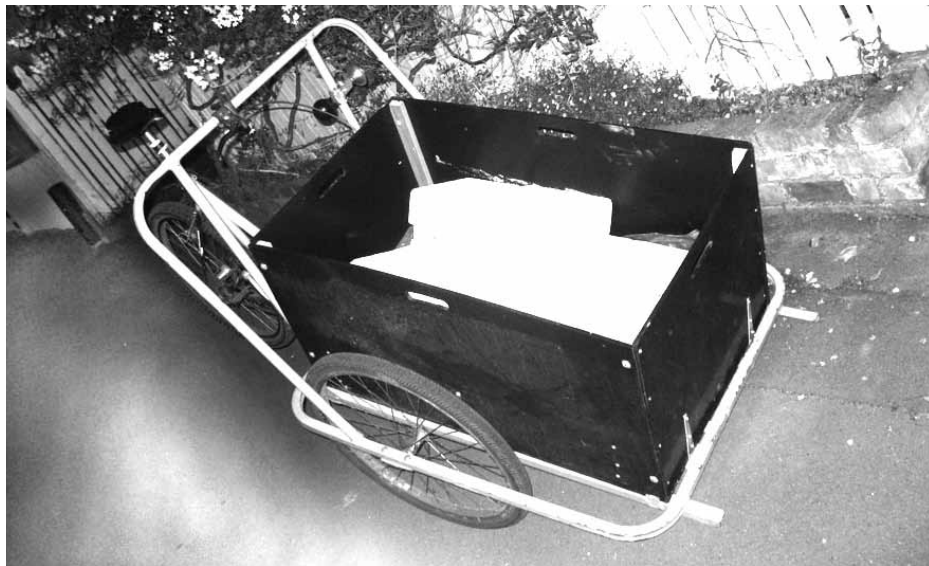
'Tadpole' three wheeled trailer loaded with 120kg of Oamaru stone
